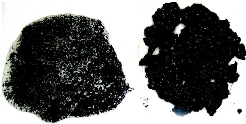
Waste Water before Separation (incl.Polymer): without with FlocFormer
